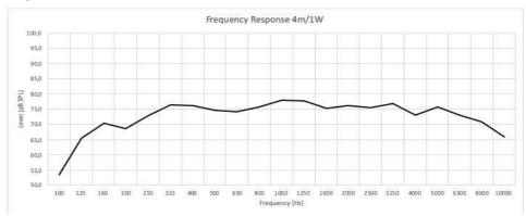
Active Eq. applied: +1,1dB@630Hz, +2dB@4KHz
